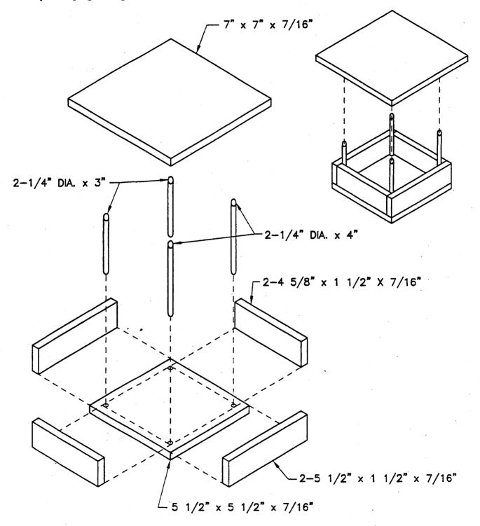
Fig. 1. Exploded view of floating shelter for 18.9-liter pitfall traps.
