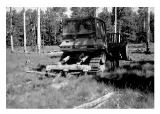
Figure 2. Severing lateral aspen roots using a tractormounted ripper. Coconino, NF, Arizona. tion with standard error bars.
